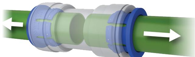
Pull on the tube to check that it is secure. It is a good practice to test the system prior to leaving site and/or before use.
