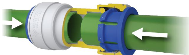
Push the tube into the tube stop. The collet (gripper) has stainless steel teeth which hold the tube firmly in position while the o-ring provides a permanent leak proof seal.
