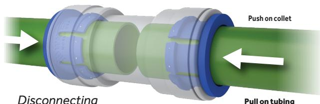
To disconnect, ensure the system is depressurized before removing the tube. Push in collet squarely against face of fitting. With the collet held in the position, the tube can be removed. The fitting can then be re-used.
